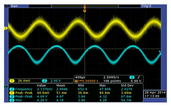
2. This is an inverting amplifier with Av = -4.07 V / 51.4 mV = -79. This is far higher gain than the measured value of Av = 4.72 without C2. But note there is already some visible distortion.
