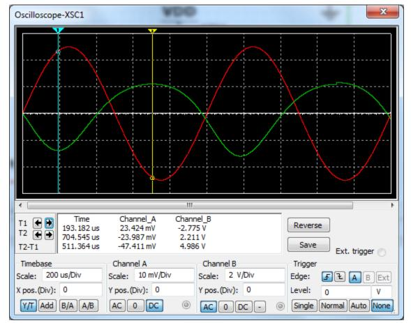
2. Simulation predicts Av = -4.986 Vpp / 50 mVpp = -99.7. But note the severe distortion.
