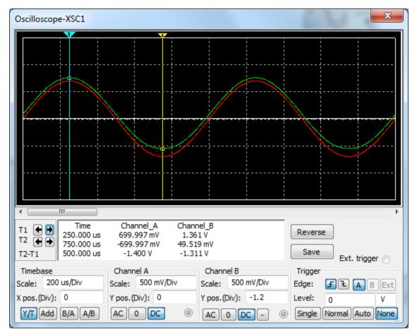
4. Continue increasing Vin until it clips on both peaks. This never happens. Shown here is with Vin = 20 Vp = 40 Vpp. The reason it never clips positive is because the transistor always maintains a constant VBE and VE < VB.
