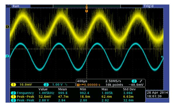
Here it is without the bypass, showing Av = 2.19 V / 43.8 mV = 50, a decrease of 16%.
