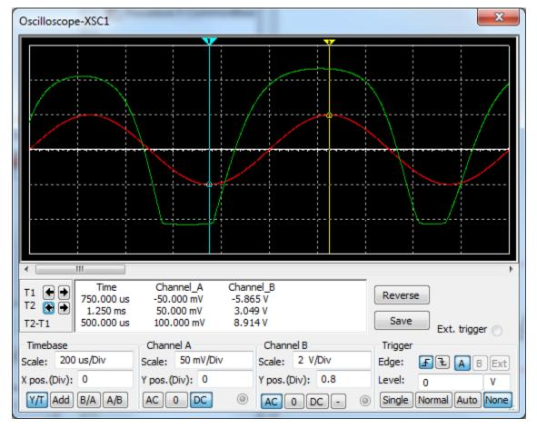
To avoid distortion, I had to reduce the input to Vin = 10 mVpp.
