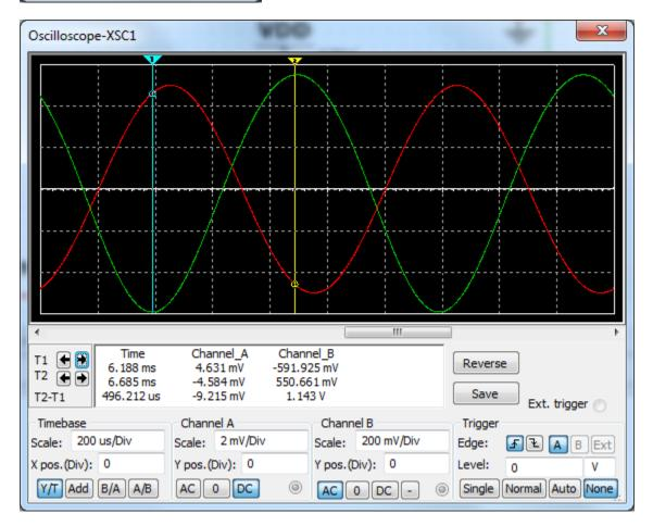
4. Clipping at both peaks occurs at Viin = 46 mVp = 92 mVpp, Vout = 8.794 Vpp.
