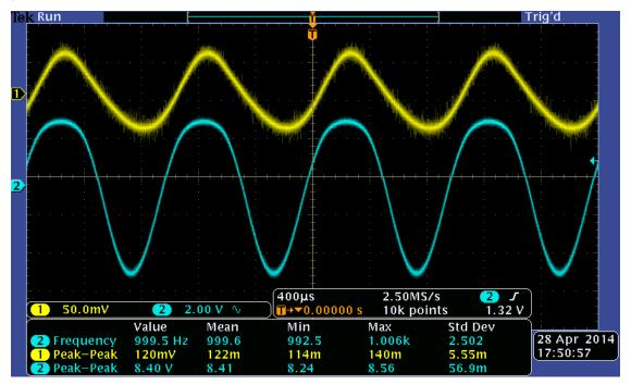
4. Increase Vin until clips both sides. Shown here, Vin = 152 mVpp, Vout = 9.47 Vpp.
