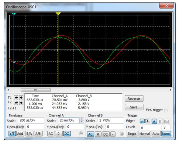
4. Clipping on both peaks at Vin = 48 mVp = 96 mVpp, Vout = 8.887 Vpp.
