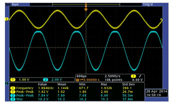
5. Increase Vin until Vout clips both peaks. Vin = 2.27 Vpp, Vout = 8.64 Vpp.
