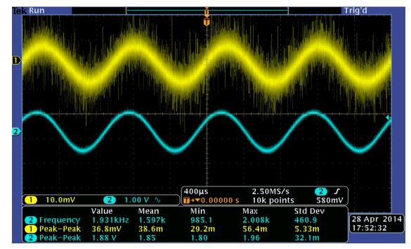
5. Reduce Vin until no clipping. Shown here, Av = 1.85 V / 38.6 mV = 48.
