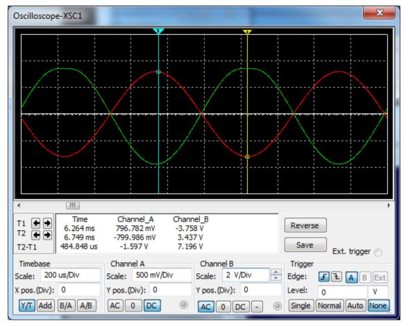
4. Clipping at the bottom happens when the transistor saturates with Vin = 1.05 Vp = 2.1 Vpp, Vout = 8.198 Vpp.
