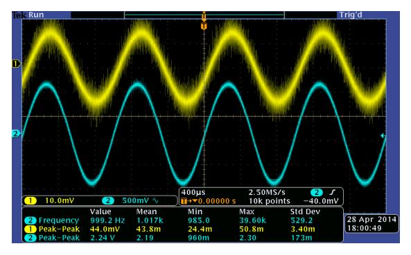
Simulation predicts a larger decrease without C1. Shown here with C1 and Vin = 20 mVpp, 1KHz, Av = 2.278 V / 20 mV = 114.
